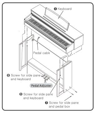
1 Place the ①keyboard on the stand and align with the holes in the side panel brackets.
